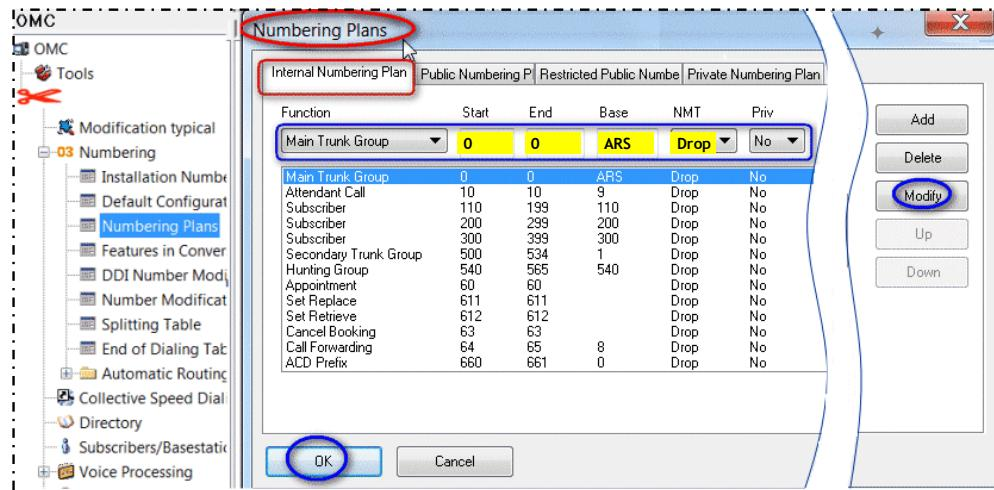
This example defines access to the internal ARS table for user dialing starting with digit 0. The "Drop" attribute indicates that the number dialed must be analyzed in the ARS Prefix table after dropping the initial digit 0.
