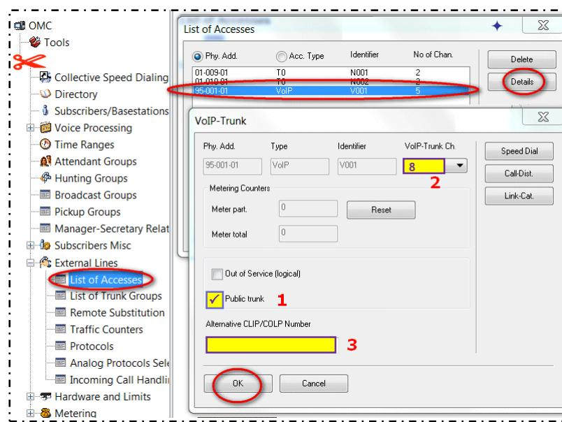
Then, configure the parameters corresponding to this VoIP Access:
