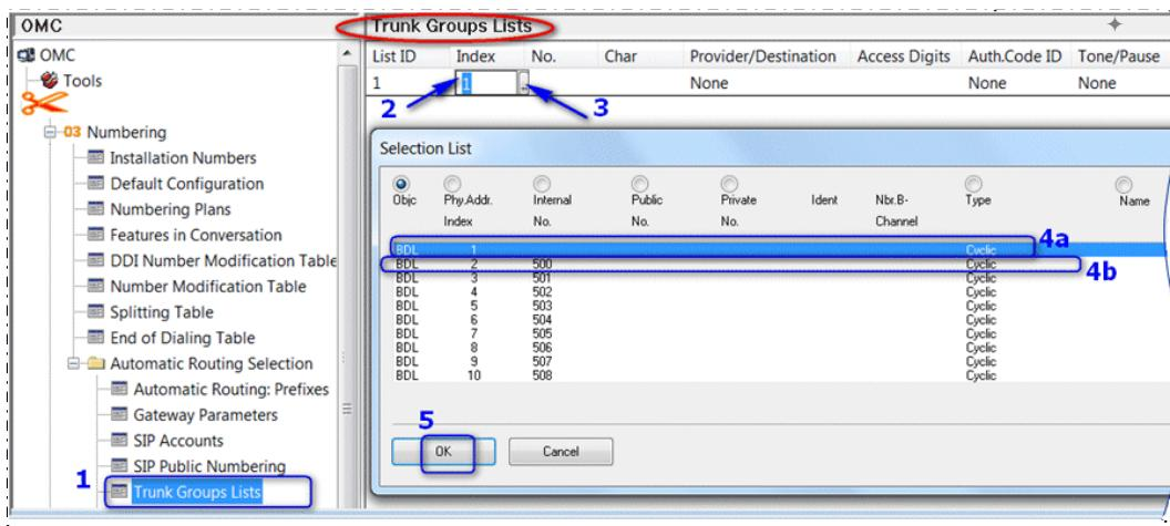
Carry out the selections and push-button steps 1 to 5 above. At step 4, you need to select the line index corresponding to the System Trunk Group previously defined at section 3.3 (i.e. action 4a for the Main Trunk Group with index #1, or action 4b for the secondary Trunk Group with index #2).
