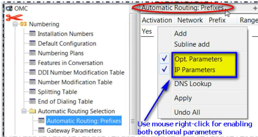
As illustrated in the following picture, you can first insert a route-line covering all type of external calls: use the Add function to create a new line and then, configure the line parameters as indicated.
