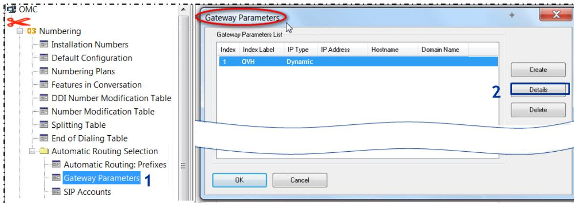
Press the button "Details" ② and then select the Domain Proxy tab of the "Gateway Parameters Details" window.
