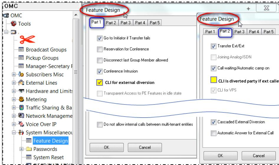
After selecting an individual extension from the menu **Subscribers/Basestation List**, use the **Details** button to access the "Feature Rights" screen and then, adjust the CLI parameter in the same way:
